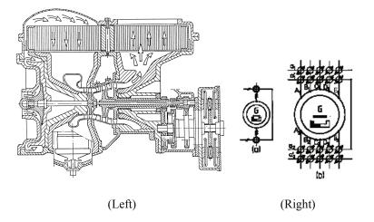
Fig. 2. The layout (left) of the automotive as turbine-generator/motor (AGT-G/M) and its (right) brushless type AC commutatorless or AC-DC/DC-AC macrocommutator magnetoelectrically-excited composite-flywheel-disc generator/motor
