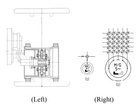
Fig. 4. The layout (left) of the road motorized and/or generatorized (RM&GW) and its (right) brushless type AC commutatorless or AC-DC/DC-AC macrocommutator magnetoelectrically-excited and reluctance in-wheel-hub motor/generator
