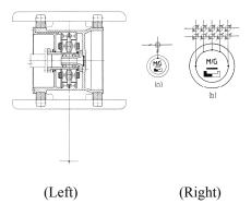
Fig. 3. The layout (left) of the sprocket and/or tensioner motorized and/or generatorized (SM&GW & TM&GW) and its (right) brushless type AC commutatorless or AC-DC/DC-AC macrocommutator magnetoelectrically-excited and reluctance in-wheel-hub motor/generator
