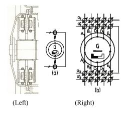
Fig. 5. The layout (left) of the brushless AC commutatorless or DC-AC/AC-DC macrocommutator IPM magnetoelectrically-excited in-wheel-hub motor/generator and its (right) electrical circuitry physical model
